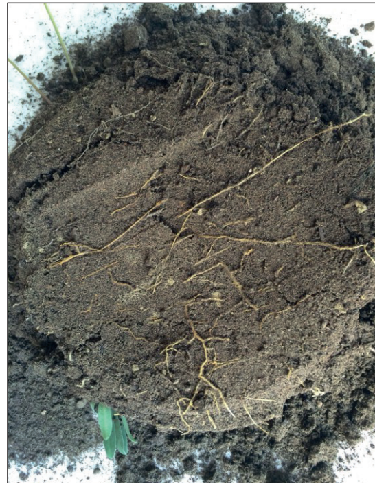
Figure 2. Typical root system at the CC5 interface after testing
