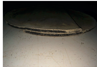
Figure 2: Joint after test. No root penetration
