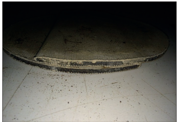
Figure 14. CC5-3 joint after the test, no root penetration
