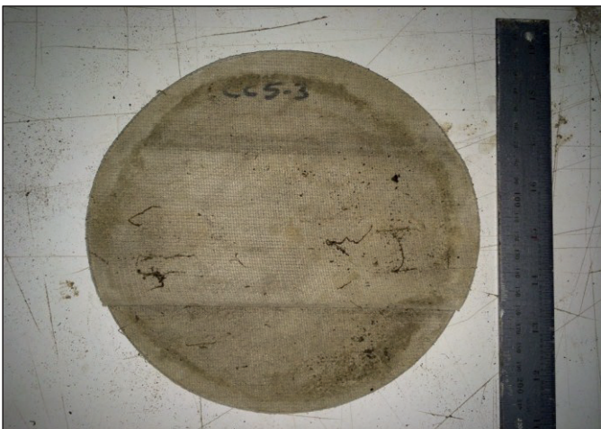
Figure 13. CC5-3 After the test (upper surface), no root penetration
