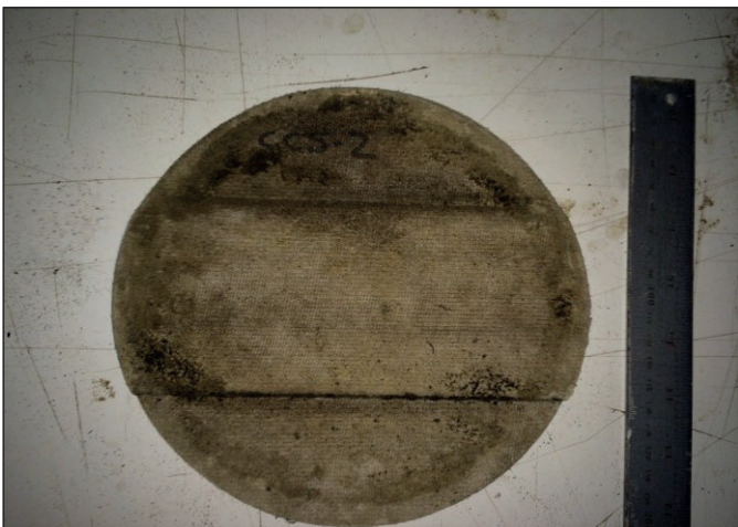
Figure 9. CC5-2 After the test (upper surface), no root penetration
